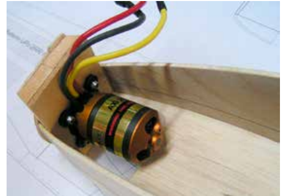
Front mount of motor 1 (Serge Delabarde).
