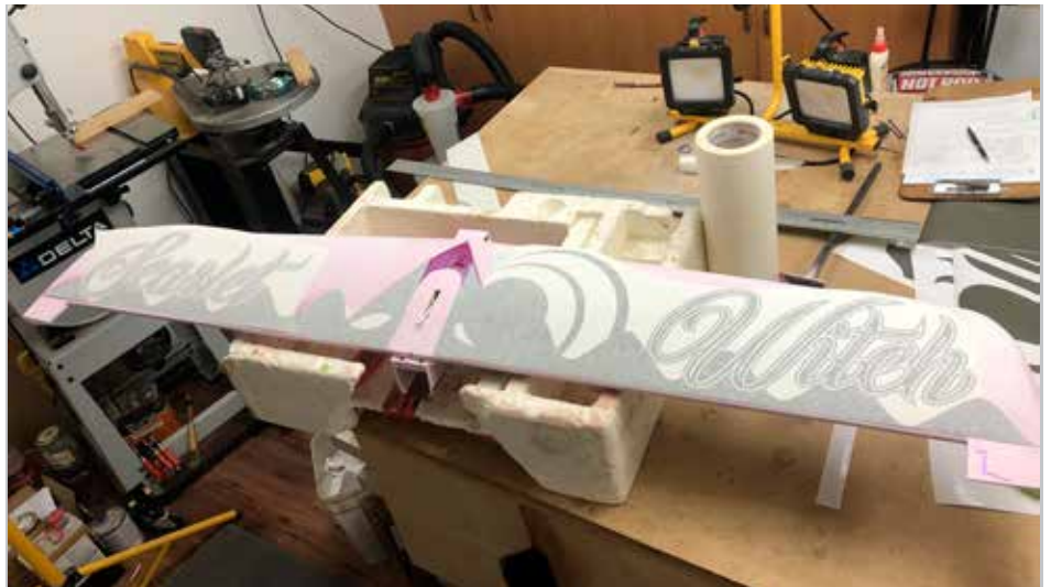
The wing has been masked with 3M vinyl. It has both shades of pink at this stage and the next color is "Pull me over Red".
