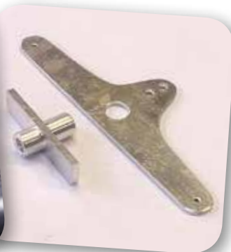
The bellcrank is made from a sheet of metal and in the center we want an axis with a diameter larger than the bolt (to get less friction). And one way is to make one in the lathe. Down to the right you can see the result.
