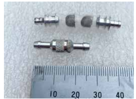
A "small" Sullivan fuel filter (top) compared to the Dub Jett filter. The later wights less than 1g.
