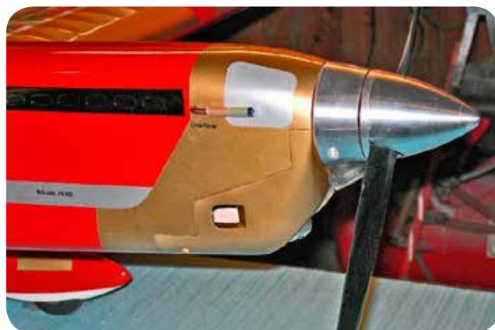
The RO-Jett .76 runs on a lightweight aluminum pipe. Note dummy rear spinner simulating the counter rotating system of the original aircraft
