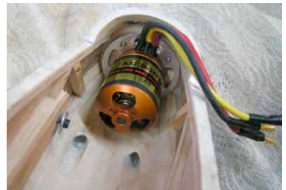
Front mount of motor 2 (Serge Delabarde).
