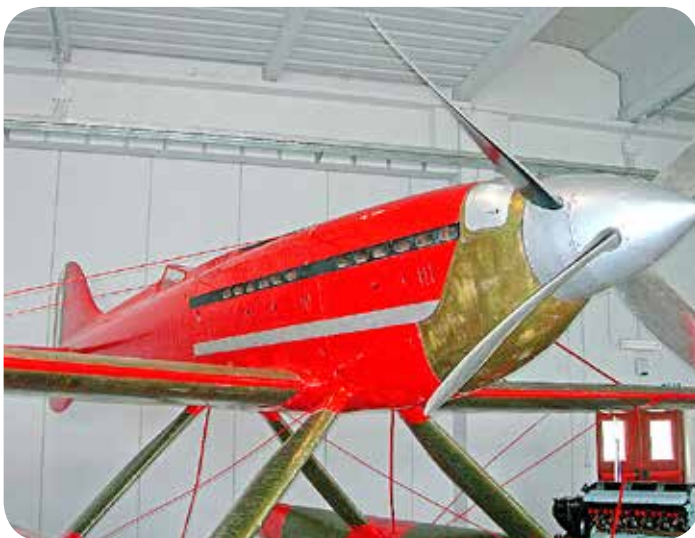
Macchi-Castoldi MC-72 had contra-rotating propellers and is a current World Record holder in its class.
