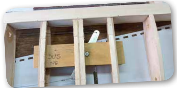
Now it is time to mount the bellcrank and before it is put in place you attach the lead-outs. They can be made from either piano wire or multi-strand wire. Also note that the front balsa strip in the leading edge is covered with balsa on all sides forming a box (the front carbon tubing is actually inside this box).
