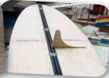
Use a plastic horn or make one in plywood.
