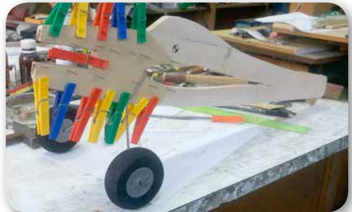
The landing gear is mounted before you attach the wing. To reinforce the front of the fuselage we glue 2 mm plywood on each side.
