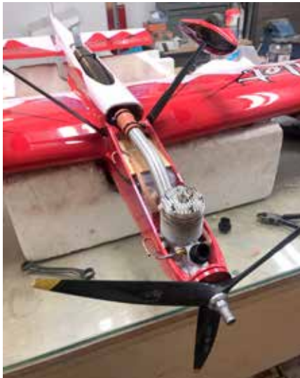
The Mighty PA75 tucks in nicely. You can see the Sullivan RST 8 flexible tank and the plug in landing gear.
