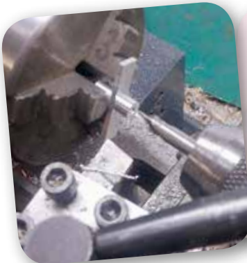
The bellcrank is made from a sheet of metal and in the center we want an axis with a diameter larger than the bolt (to get less friction). And one way is to make one in the lathe. Down to the right you can see the result.
