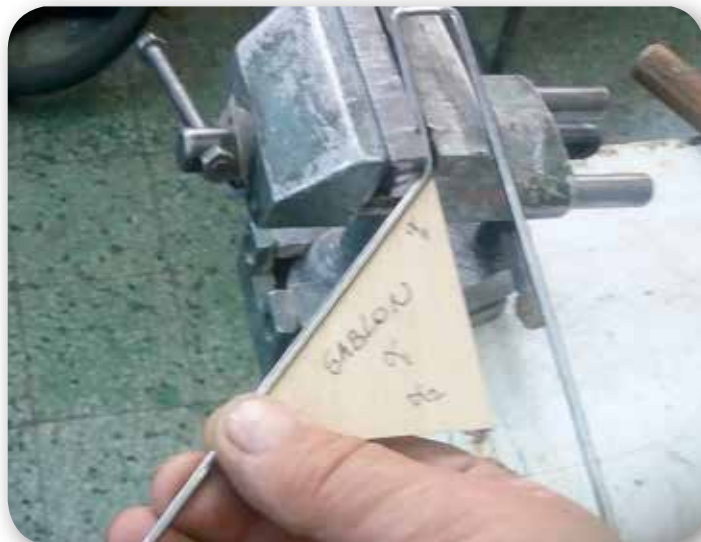
Landing gear is made from 3 mm piano wire and bent in a vise. Use templates to get correct angles. If you succeed it should look like the one on the photo to the right.
