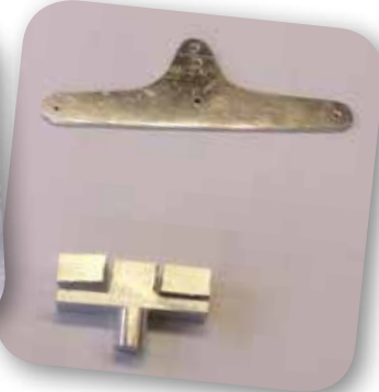
The bellcrank is made from a sheet of metal and in the center we want an axis with a diameter larger than the bolt (to get less friction). And one way is to make one in the lathe. Down to the right you can see the result.
