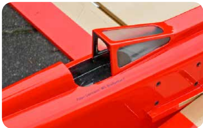
The open frame canopy is not easy to build and difficult to paint neatly.
